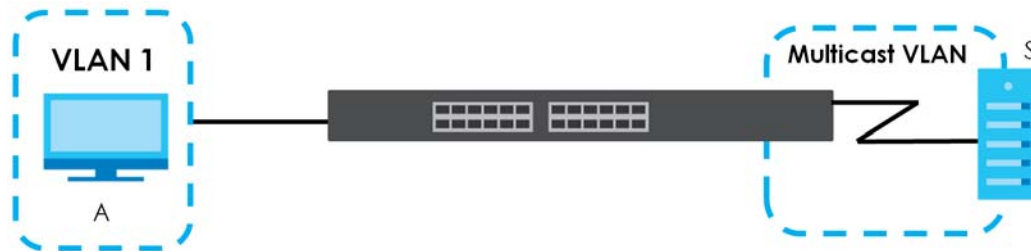
Figure 151 MVR Multicast Television Example
